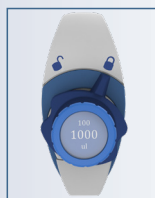
Volume lock to prevent unintended volume adjustments
