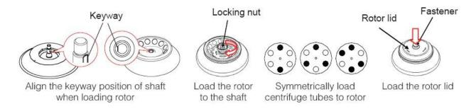
Figure 8-2 the rotor installation
