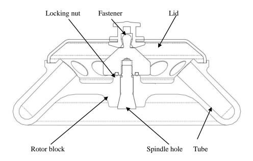
Figure 11-1 the rotor profile
