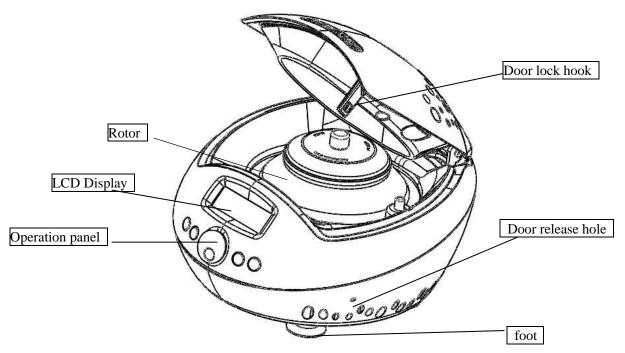
Figure 5.1 Front view of centrifuge
