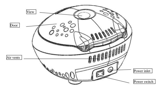
Figure 5.2 Rear view of centrifuge
