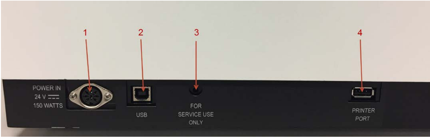
Rear ports on a reader with incubation capability
